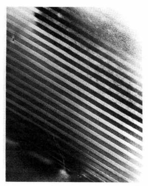
COMPUTER-ENHANCED detail of transmission electron micrograph showing individual layers of strained-layer superlattice (SLS) structure. Shades of gray along length of layers have been averaged out by electronic processing.
